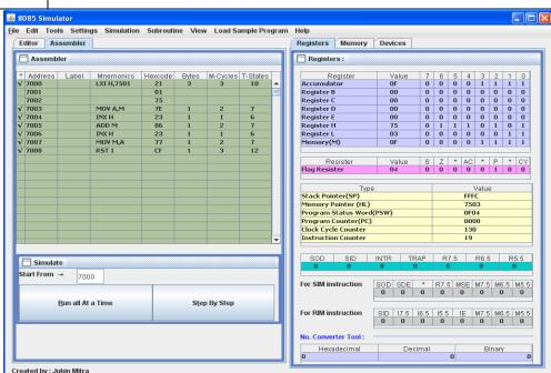
Simulation using Open Source Tool – 8085 Simulator
